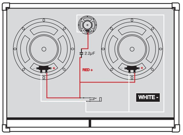
= Capacitor for blocking low frequencies from reaching the high frequency driver. Value 2.2µF Crossover 2kHz
